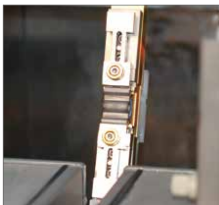
Transverse heating ensures uniform atomization of whole sample. Sample injected into the highest temperature region between graphite tube wings; both wings have large thermal mass, therefore with maximum heat conductivity, would heat the sample uniformly.
