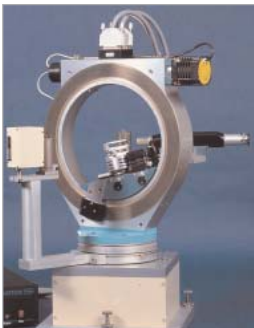
Difftech Texture Automation fitted to a Huber Texture Circle mounted on a harmonic gearbox base goniometer
